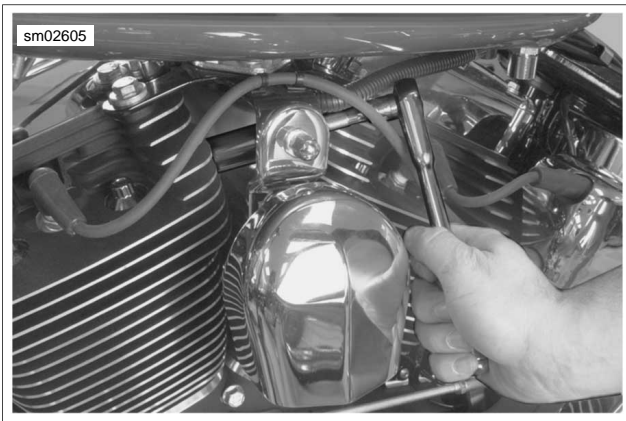
Figure 4-16. Engine Temperature Sensor Removal
