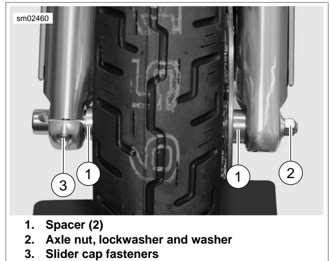
Figure 2-8. Front Axle Assembly
