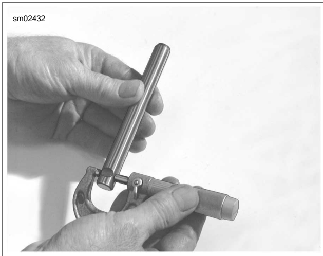
Figure 3-77. Checking Shaft to Support Plate Fit
