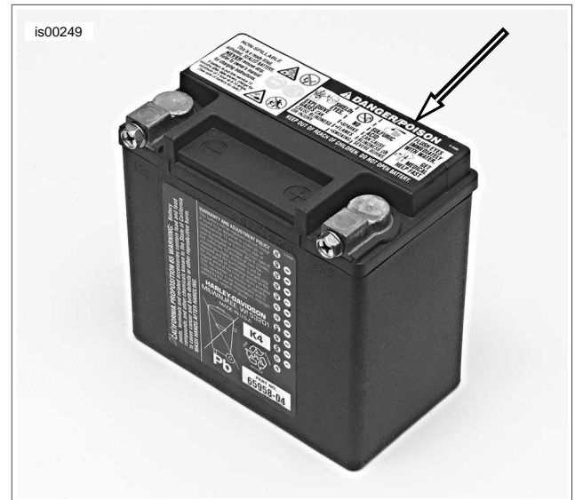
Figure 1-37. AGM Battery with Warning Label
