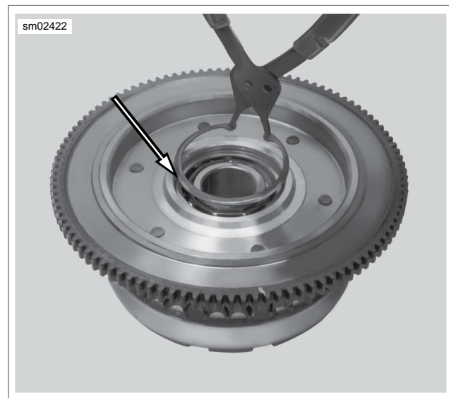
Figure 6-34. Install Clutch Shell Retaining Ring with Flat Side Against Bearing
