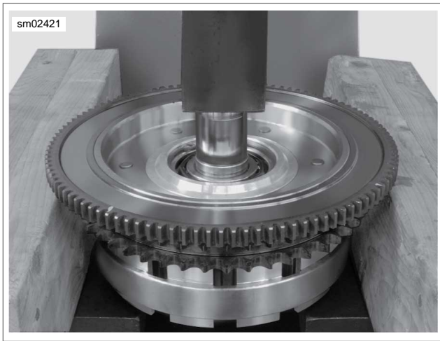
Figure 6-33. Pressing Clutch Hub From Bearing
