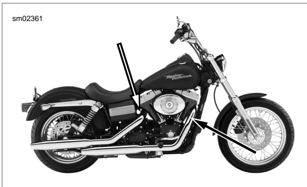
Figure 4-27. Oxygen Sensors (Inboard Side of Exhaust Pipes)
