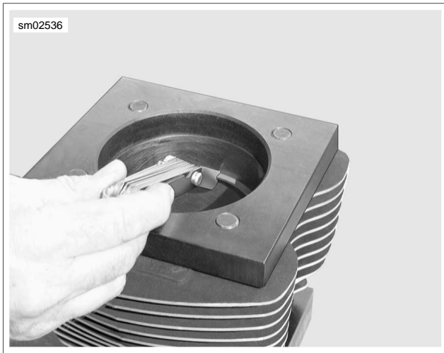
Figure 3-109. Measuring Ring Gap
