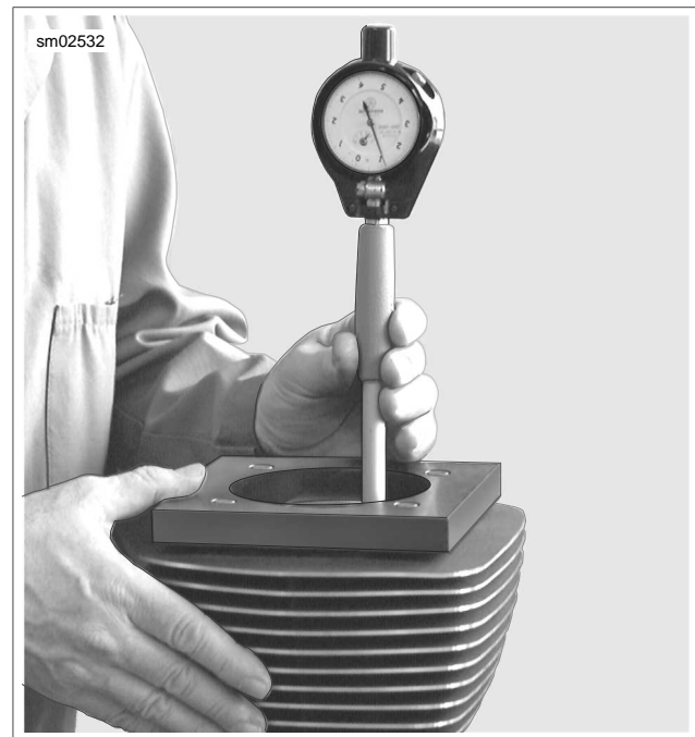
Figure 3-104. Measure for Out-of-Round and Taper
