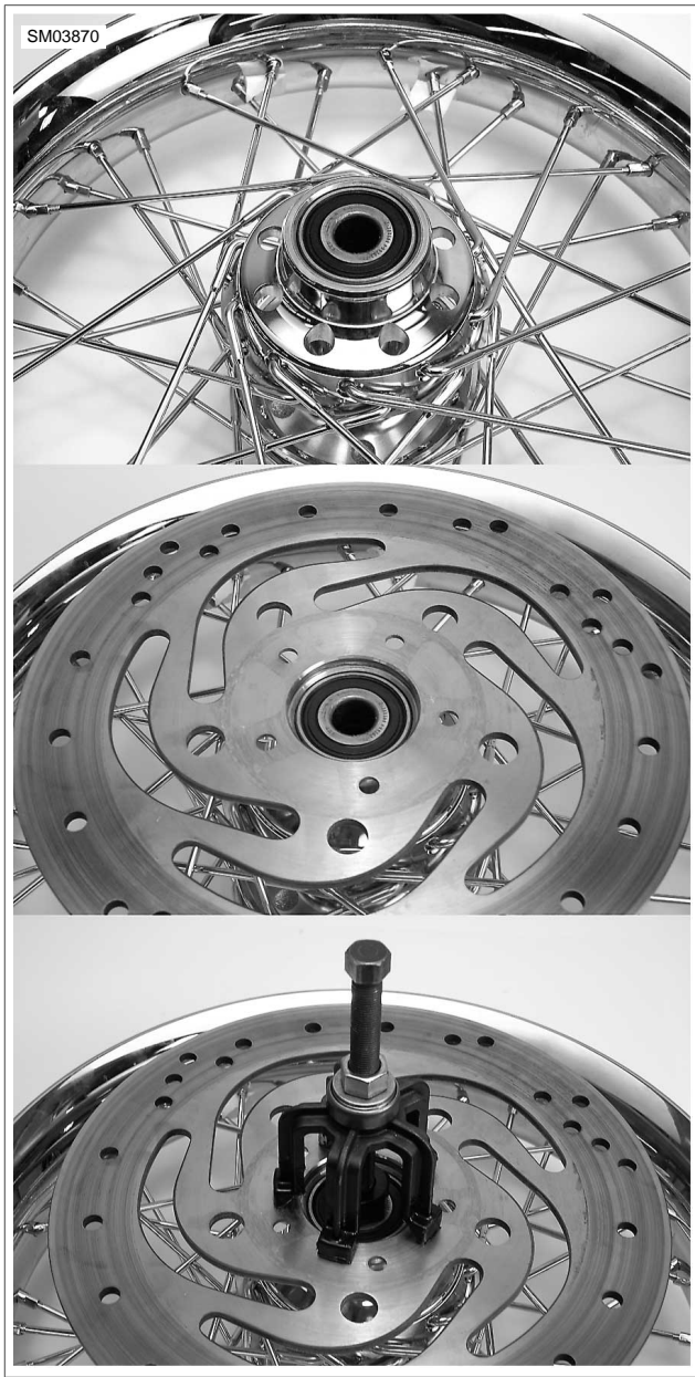
Figure 2-15. Brake Disk as Puller Aid
