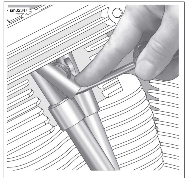
Figure 3-48. Install Spring Cap Retainers
