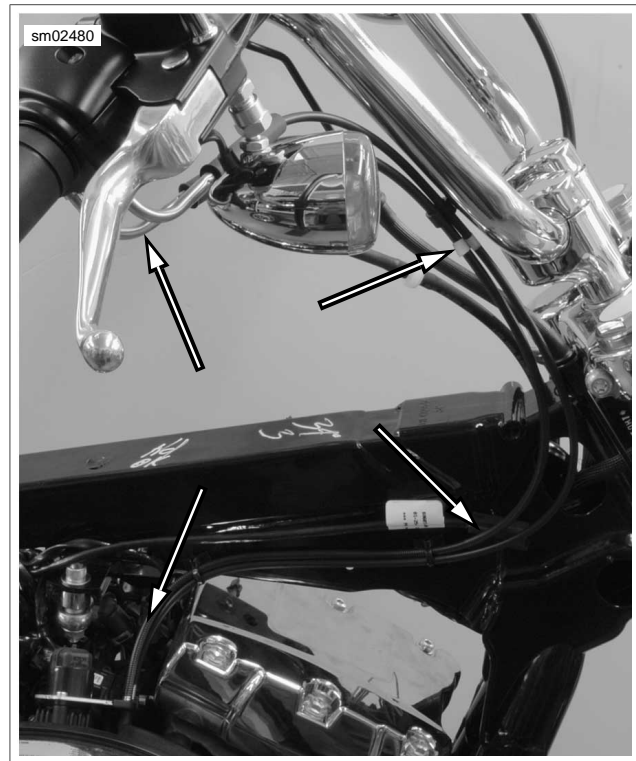
Figure 2-96. Throttle Cable Routing: FXDWG, FXDF (Typical)
