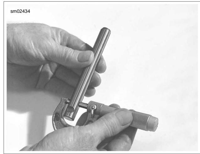
Figure 3-79. Checking Shaft to Bushing Fit
