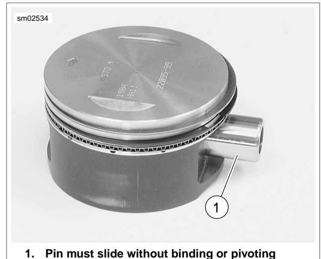
Figure 3-106. Piston Pin Clearance
