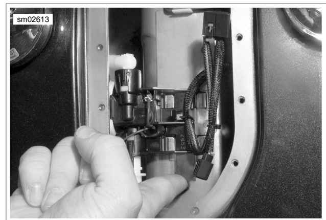
Figure 4-39. Fuel Pump Removal
