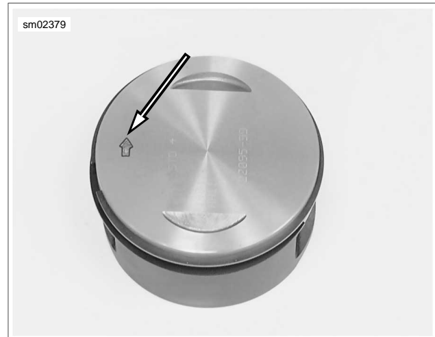
Figure 3-30. Piston Installation Arrow
